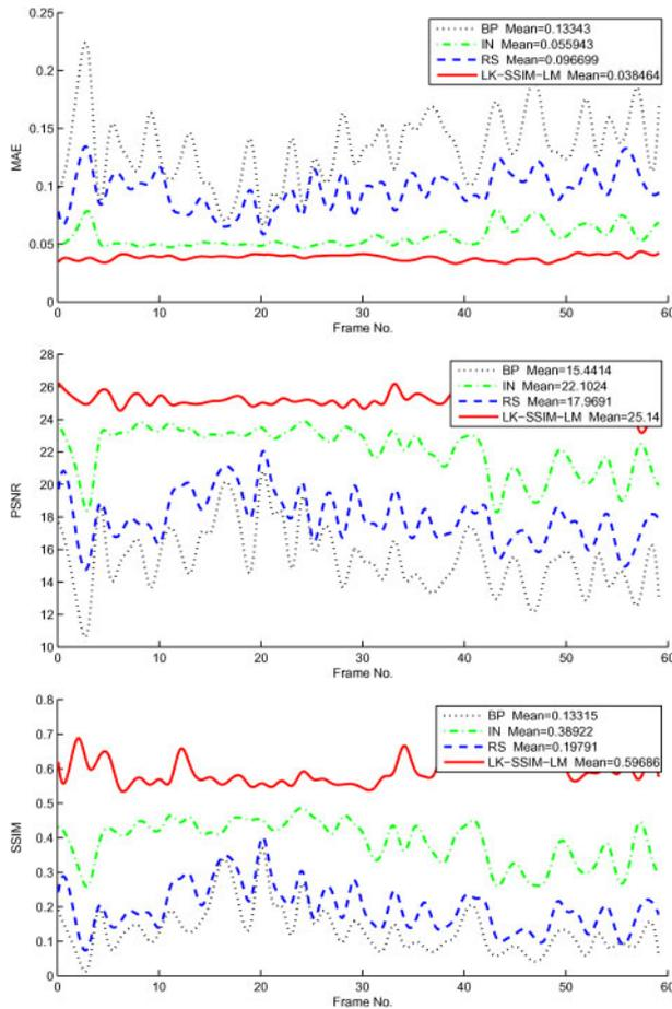
**5** MAE, PSNR and SSIM comparison of the proposed video enhancement algorithm (Algorithm 2) and some super-resolution reconstruction methods for ‘Tokyo’ sequence
