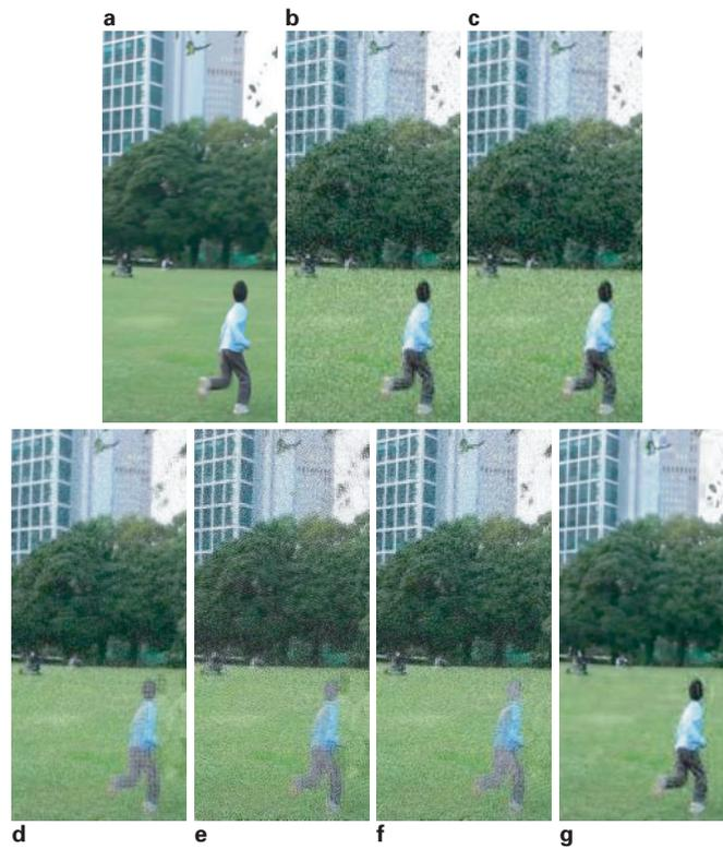
6 Close-up views of the original HR image, replication (nearest) and bicubic resizing methods, and super-resolution reconstruction methods: interpolation, iterated back-projection<sup>13</sup> robust super-resolution<sup>31</sup> and the proposed method in Algorithm 2 on ‘Tokyo’ sequence: (a) original HR frame; (b) LR frame (nearest); (c) LR frame (bicubic); (d) interpolation; (e) iterated back-projection; (f) robust super-resolution; (g) this paper
