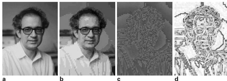
2 Comparing the error maps of two images based on MSE and SSIM. The images are taken from Ref. 8: (a) original image; (b) JPEG compressed; (c) MSE map; (d) SSIM map
