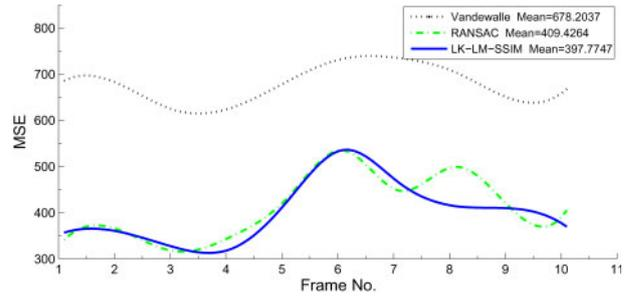
9 Reconstruction error, when some other registration methods are used in Algorithm 2, instead of 'LK-LM-SSIM'
