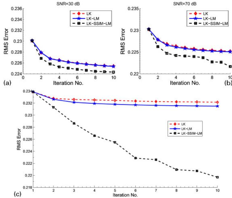
3 Convergence comparison of the proposed LK-SSIM-LM algorithm and two other variations of LK algorithm for ‘Tokyo’ sequence: (a) LR images: SNR=30 db; (b) LR images: SNR=70 db; (c) mean RMS over all experiments for SNRs=20, 30, 50 and 70 db
