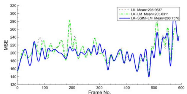
4 MSE comparison of the proposed video enhancement algorithm (Algorithm 2) using different variations of LK algorithm for ‘Tokyo’ sequence
