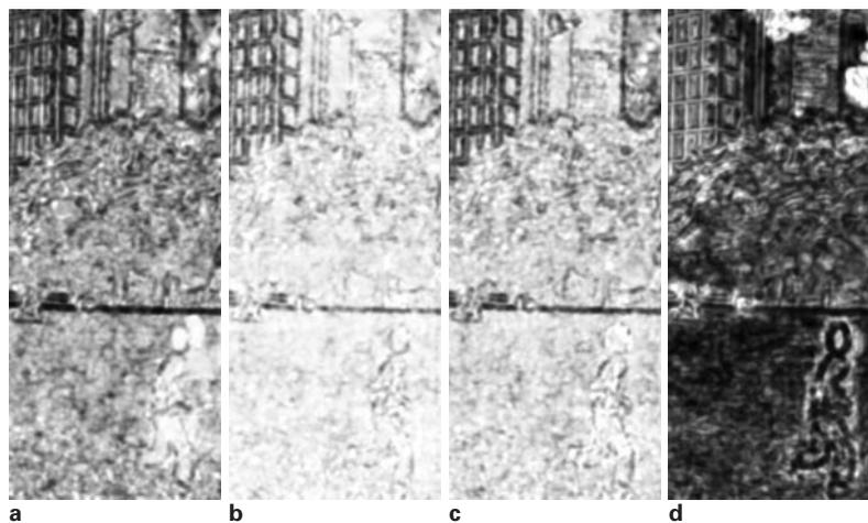
7 SDIS map image ( $E_{SDIS}$ ) between Fig. 6d-g with related HR image (Fig. 6a). Brighter pixel means higher error: (a) interpolation; (b) iterated back-projection; (c) robust super-resolution; (d) this paper
